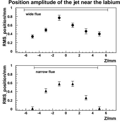
Figure 3: Jet amplitude at 5 mm from the flue exit as a function of  $Z$  (geometrical width is indicated).
