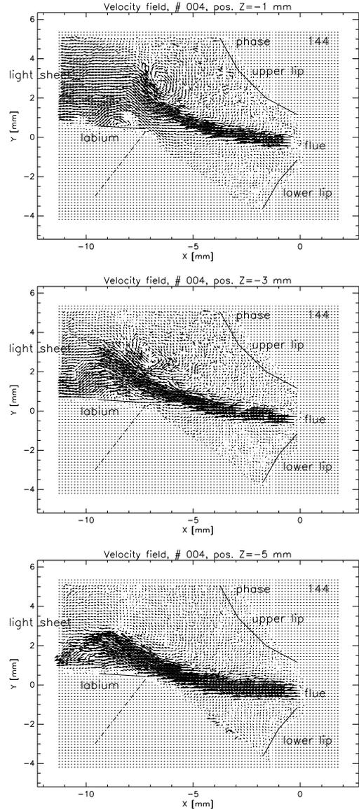
Figure 2: Velocity fields. Top, middle, bottom: at position  $Z = -1 \text{ mm}$ ,  $-3 \text{ mm}$ ,  $-5 \text{ mm}$  off center, respectively.
