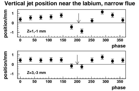
Figure 6: Jet position at 5 mm from the flue exit as a function of the phase for the narrow flue.
