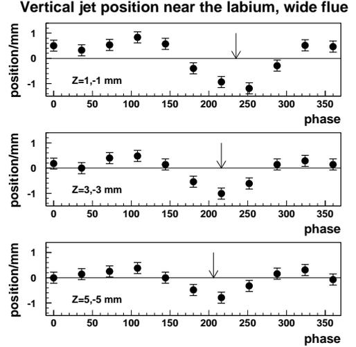
Figure 5: Jet position at 5 mm from the flue exit as a function of the phase for the wide flue.
