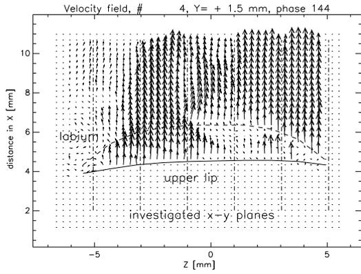
Figure 4: Velocity field of the wide flue viewed from top.
