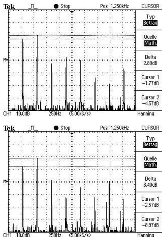
Figure 1: Spectral distribution of the pressure amplitude: above 12.5 mm flue, below: 9.5 mm flue.
